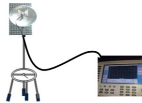
Gambar 3. Set up pengukuran VSWR
