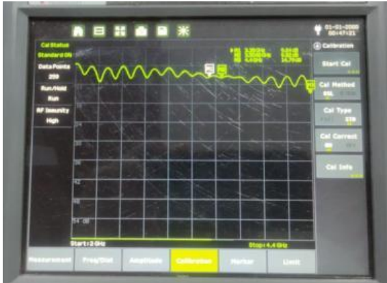
Gambar 4. Return Loss Terminator 5x3x3 cm
