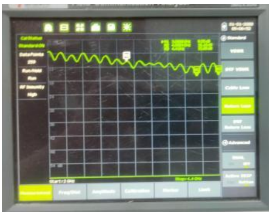
Gambar 10. Return Loss Terminator 20x3x3 cm
