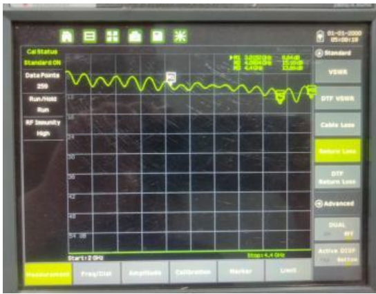
Gambar 8. Return Loss Terminator 15x3x3 cm
