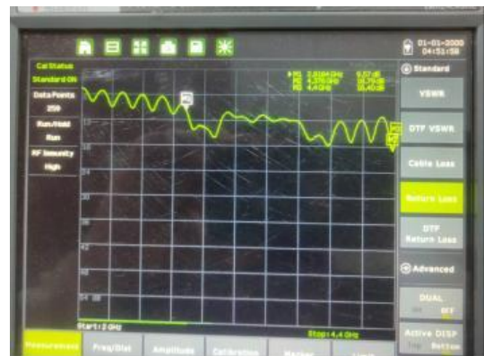
Gambar 12.. Return Loss Terminator 25x3x3 cm
