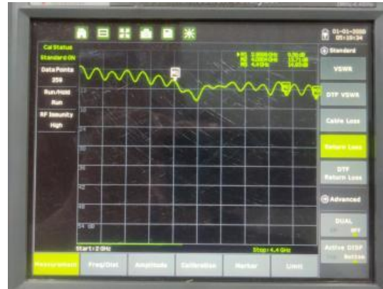
Gambar 6. Return Loss Terminator 10x3x3 cm
