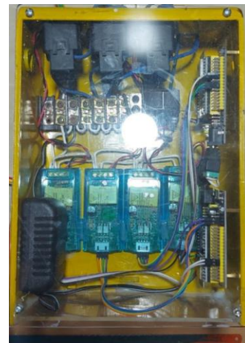
Gambar 3. Design Alat Monitoring Arus dan Tegangan
