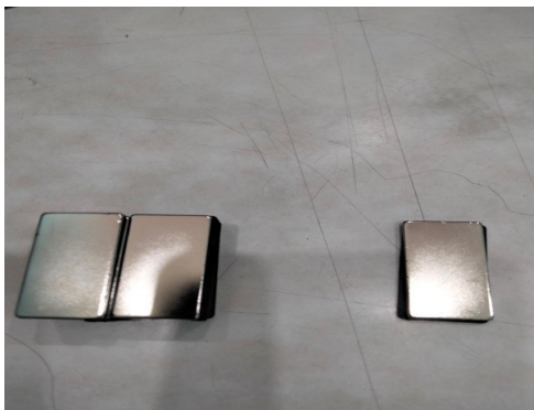
Gambar.8. Magnet neodymium Nd2Fe14B
