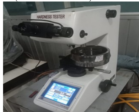
Gambar 1. Mesin Jominy Test (Microhardness Vickers)
