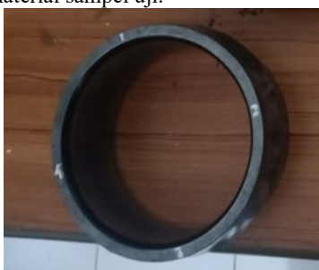
Gambar 3. Sampel uji Roll Bearing (inner bearing)
