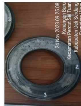
Gambar 4. Sampel uji Taper Bearing (inner bearing)
