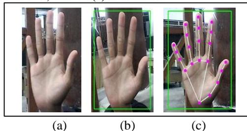
Gambar 6 Proses single shot detector dan landmark
