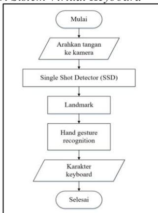
Gambar 3 Flowchart Sistem Virtual Keyboard
