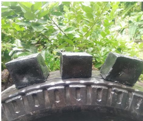
Gambar 2. Paving block 100% berbahan plastik
