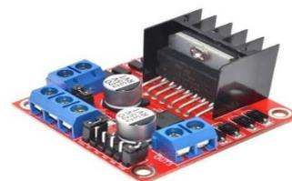
Gambar 5. Modul Motor Shield L298N
