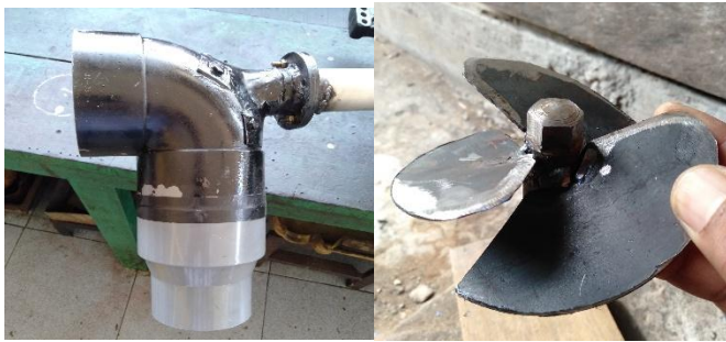
Gambar 9. Propeller water jet outboard
