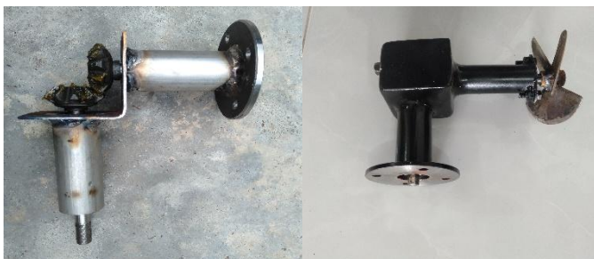
Gambar 10. Gear box baling- baling Konvensional Biasa
