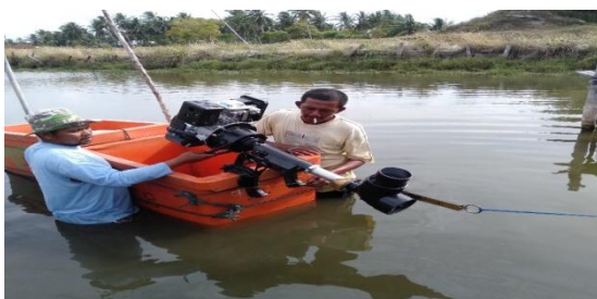
Gambar 17. Pengujian Propeller Water Jet Propulsion
