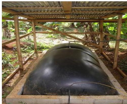
Gambar. 3 Tipe Digester Baloon Plant
