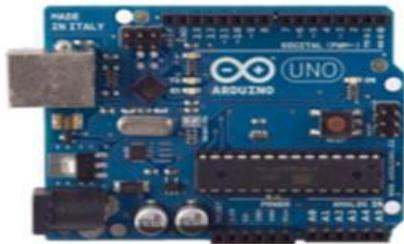
Gambar 3. Modul Arduino Uno
