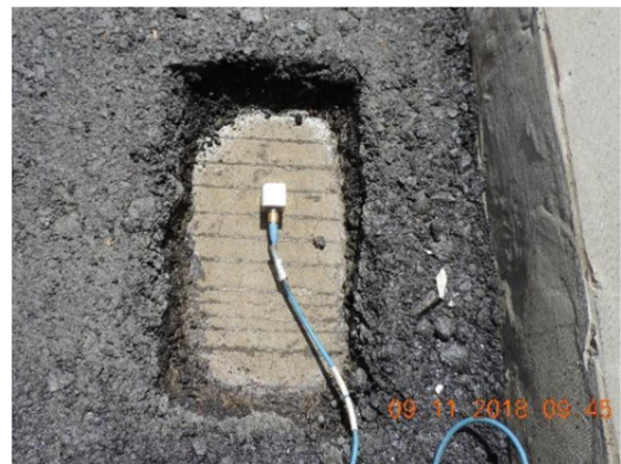
Gambar 7. Sensor accelerometer (PT. Risen Eng. Consult, 2018)
