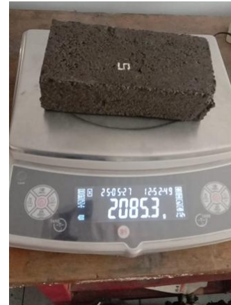
Gambar 4. Penimbangan paving block kondisi JPK
