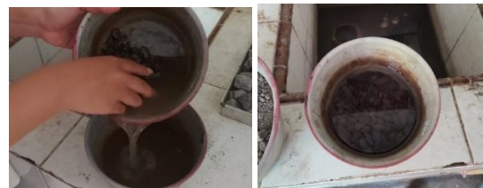
Gambar 4. Proses pengujian kadar lumpur
