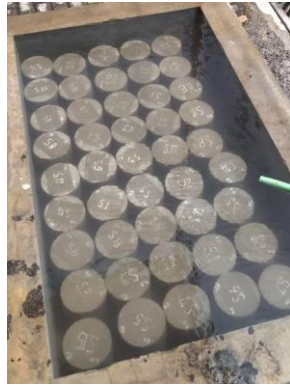
Gambar 10. Proses perendaman beton
