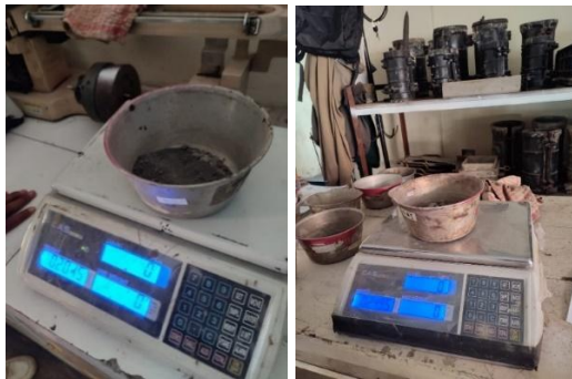
Gambar 2. Proses pengujian kadar air
