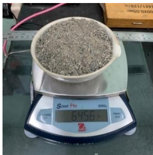
Gambar 6. Pengujian kadar air agregat halus
