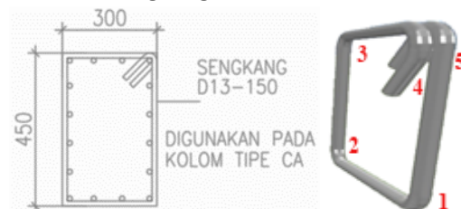
Gambar 4. Besi Sengkang Kolom CA
