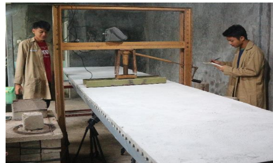
Gambar 21. Uji Model PGU Orthotropic Composite
