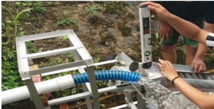
Fig. 1. Experimental setup showing the mounting of the Archimedes screw turbine, flow direction, and adjustable frame components
