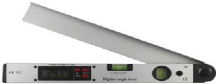
Fig. 2. Close-up view of the digital angle level used to set turbine inclination precisely
