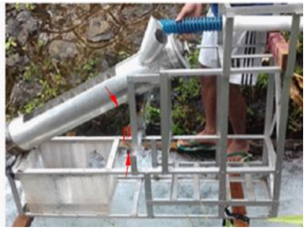
Fig. 1. Experimental setup showing the mounting of the Archimedes screw turbine, flow direction, and adjustable frame components
