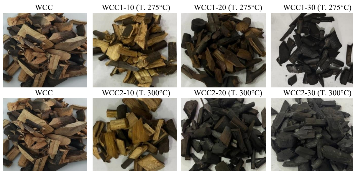
Fig. 4. Visual torrefaction result of Calliandra wood chips
