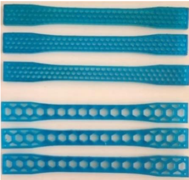
Fig. 9. SLA Results of honeycomb specimens with ratios of 5 mm and 10 mm
