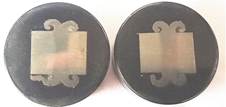
Fig. 6. Cross section of RFW joints JIS S45C, as-weld (left side); stress relieving (right side)
