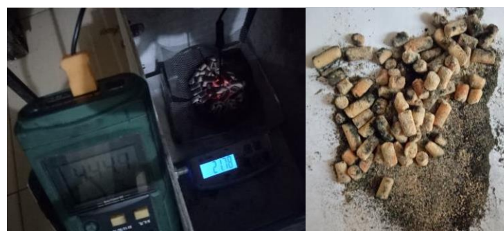
Fig. 6. Combustion Rate (a) Bio-pellets during combustion (b) Bio-pellets after combustion
