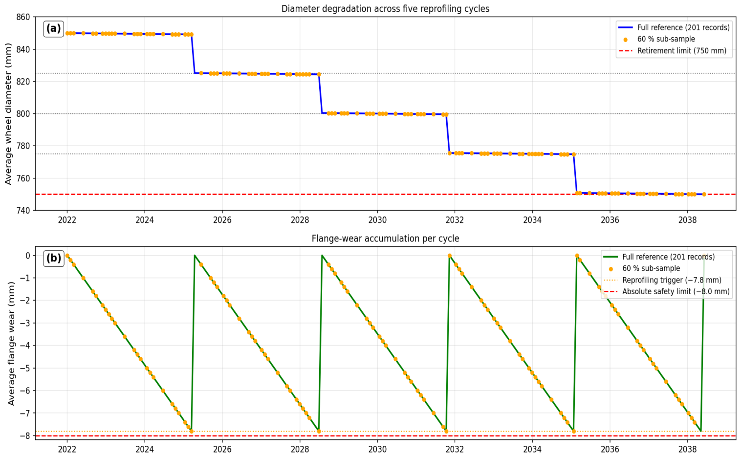
Fig. 1. Wheel diameter degradation (a) and flange wear per cycle (b) across the full 16.4-year life.
