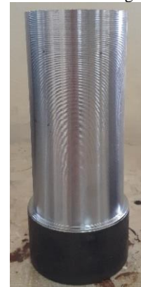
Fig. 3. Aluminium Al-6061 AlMgSiCu test material
