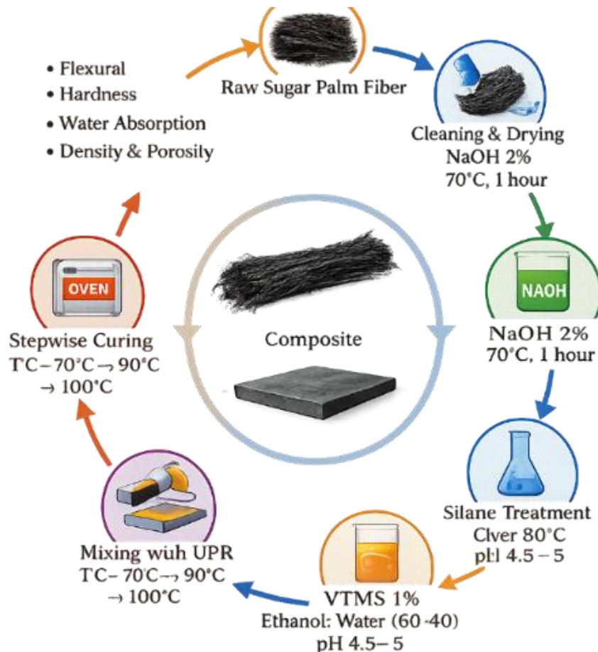
Fig. 1. Schematic illustration of alkali-VTMS treatment of sugar palm fiber and composite fabrication.
