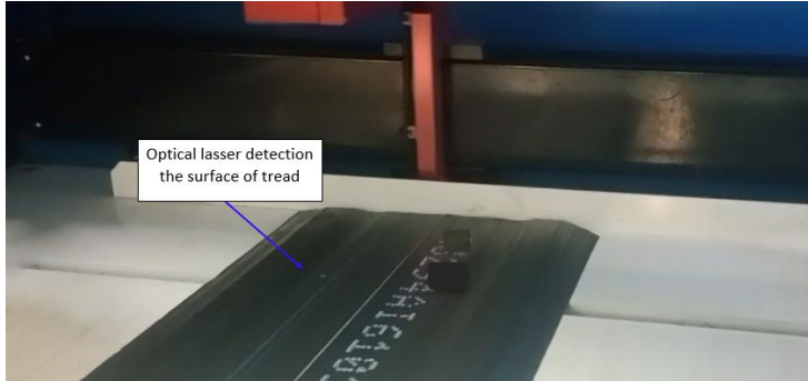
Fig. 6. Optical laser profilometer scanning process on the tread.
