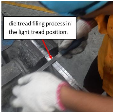
Fig. 11. Repair process of tread die.
