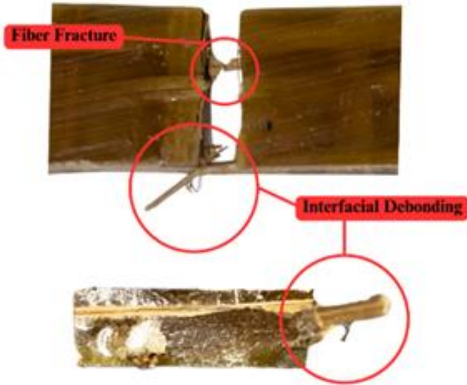
Fig.11. The macroscopic fracture observations of specimen 70E30SB 0% B 4 C after tensile test
