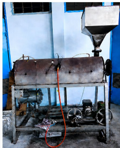
The main components of the reactor comprise the reactor tube (1), biomass feed hopper (8), drive system (electric motor and gear reducer) (2,3), LPG burner as the heat source (9), temperature recording system (data logger with K-type thermocouple sensor) (4), cooling-char system (5,7,10), and torrefaction product collection container (6).
