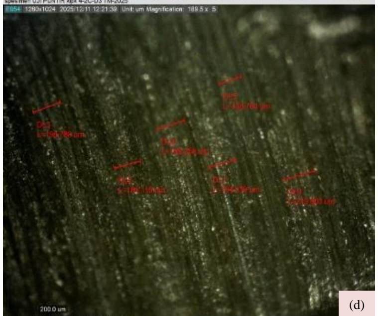
Fig. 7. Plates thickness 2 mm macro burr defect measurement. (a) 400 rpm depth cut 0.25 mm, (b) 400 rpm depth cut 0.5 mm, (c) 800 rpm depth cut 0.25 mm, (d) 800 rpm depth cut 0.5 mm.
