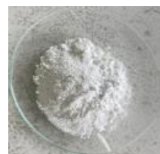
Fig. 3. Synthesized hydroxyapatite powder obtained via green synthesis.
