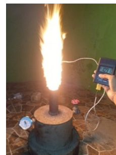
Fig 6. Water steam stove testing
