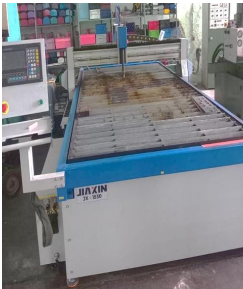
Fig. 3. CNC plasma cutting JIAXIN JX-1530 machine
