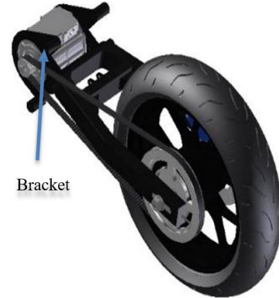
Fig. 4. BLDC support bracket for electric vehicles
