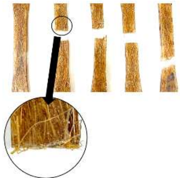
Fig. 6. Tensile test results of untreated specimens
