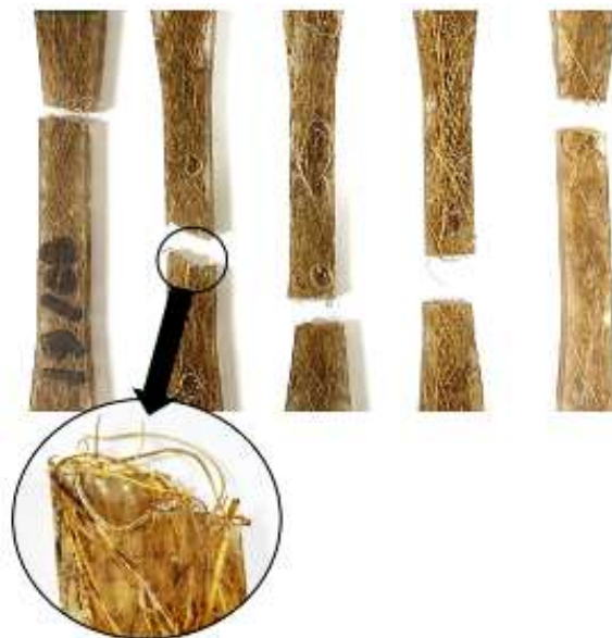
Fig. 9. Tensile test results of 10% NaCl-treated specimens
