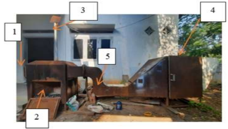
Fig. 8. Coffee bean drying machine
