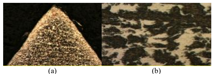
Fig. 3. Microstructure of core area 500× magnification (a) sample A1, (b) thread area 50× magnification with 3% nital etching.
