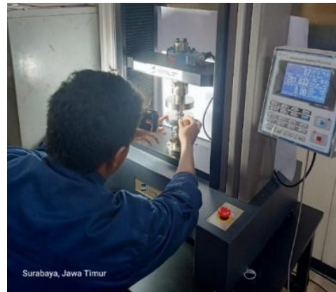
Fig.13. Quasi-static compression test setup using the SALT ST-1001 C UTM machine
