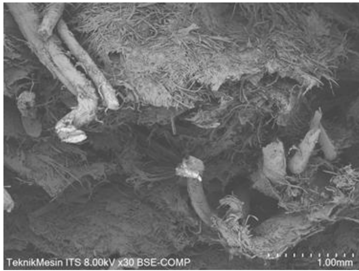
Fig. 14. Fibre and interface condition on the fracture surface from the bending test (the highest value). Fibre length: 1 cm, reinforcement weight fraction: 10%. Magnification: 30x
