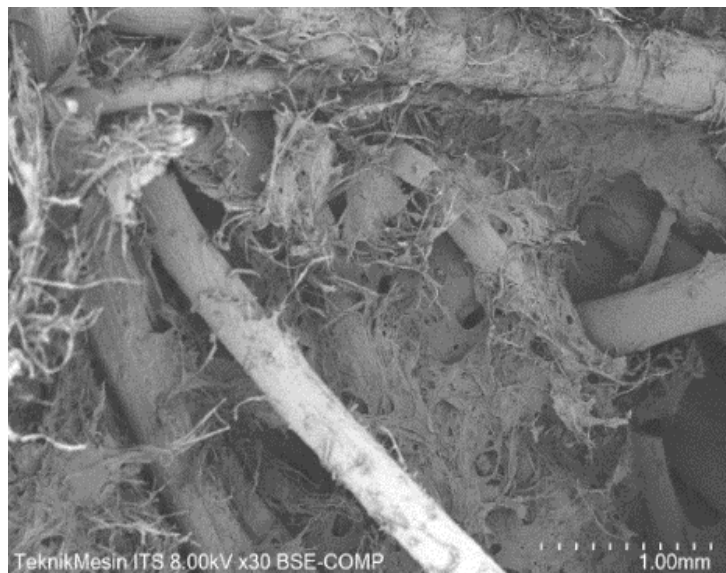
Fig. 11. Fibre condition on the fracture surface of the tensile test results (the lowest value). Fibre length 1 cm with a weight fraction of 40%. Magnification 30x
