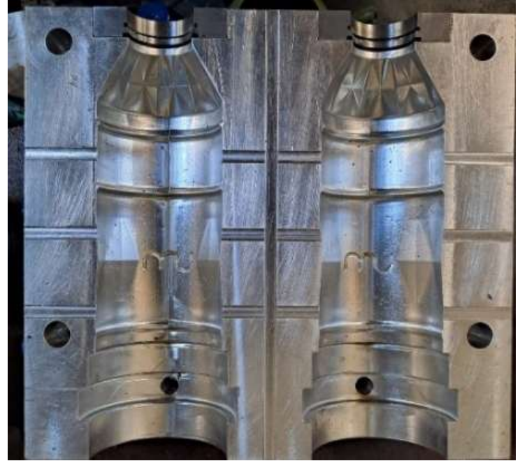
Fig. 2. Molding of the PET Product
