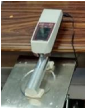
Fig.4. Procedure for measuring actual surface roughness
