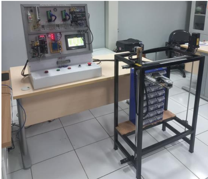
Fig. 10. Final prototype of the 3-Axis ASRS
