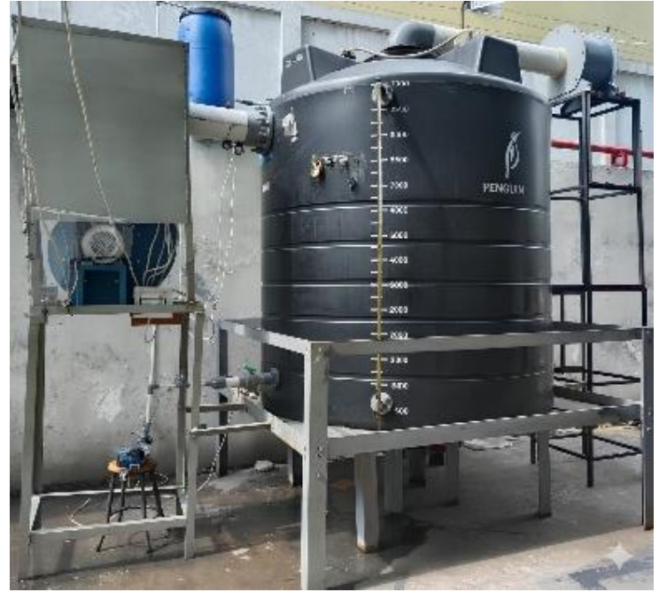
Fig. 5. Desalination reactor construction
