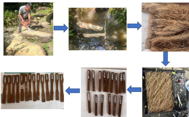
Fig. 1. Composite specimen fabrication process
