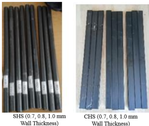
Fig. 3. CHS and SHS specimens
