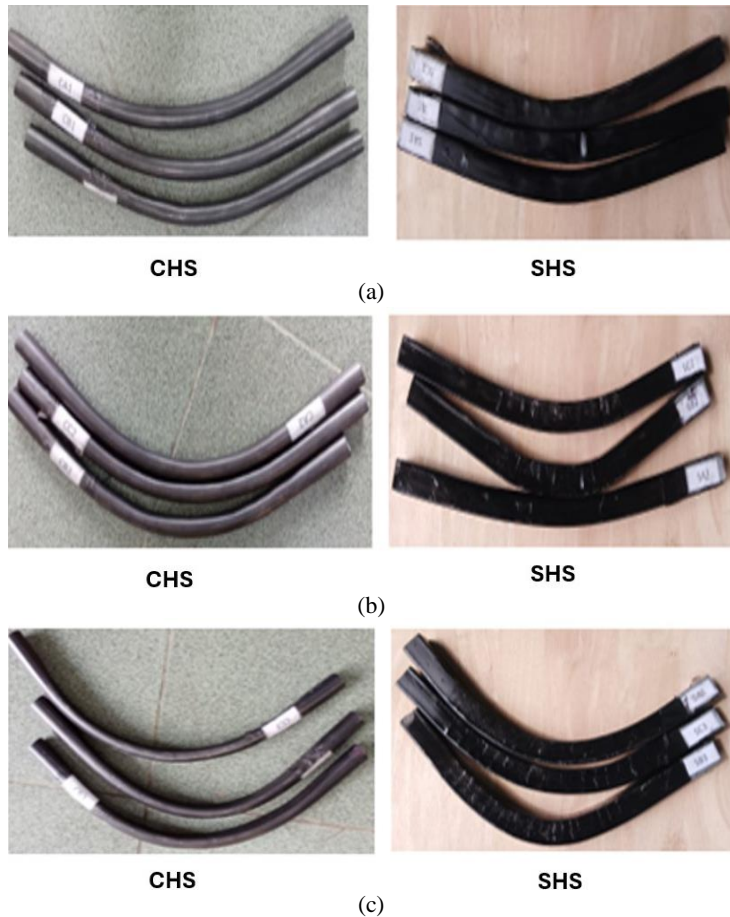
Fig. 4. Bending results: (a) 30°, (b) 60°, and (c) 90° bending angle
