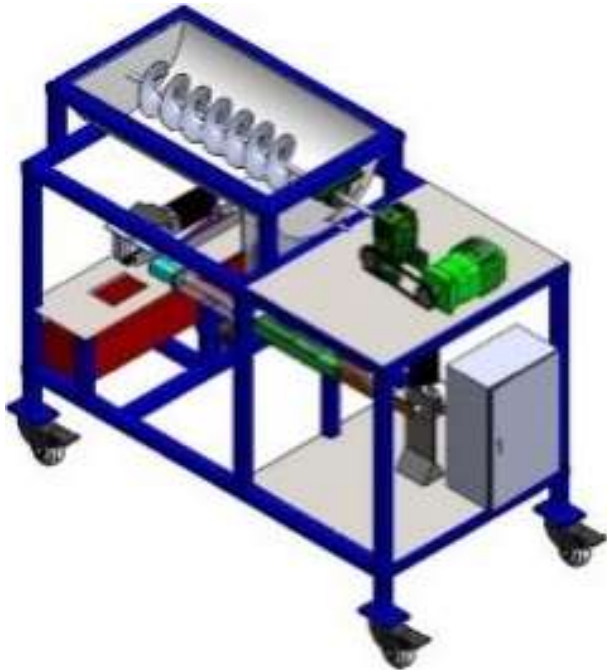
Fig. 6. Design of a mixer briquette making machine.
