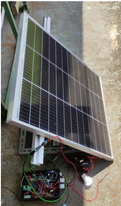
Fig. 2. Solar panel and SCC MPPT box.
