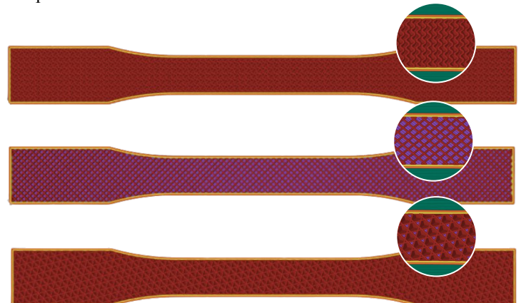
Fig. 2. Variety of infill pattern types from top to bottom: Gyroid, grid, and cubic
