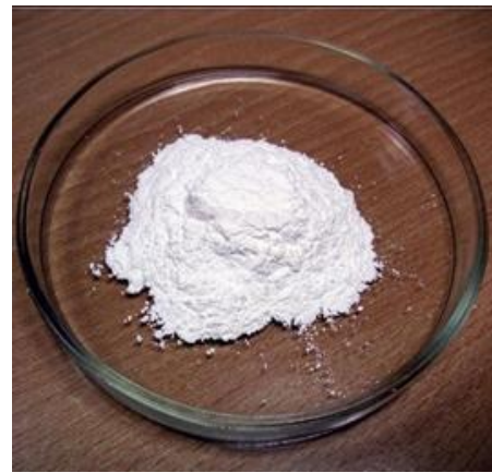
Fig.2. Bio-HA powder as a suspension material for coatings
