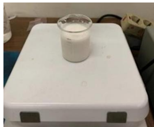
Fig.3. HA suspension for Ti-12Cr coating.
