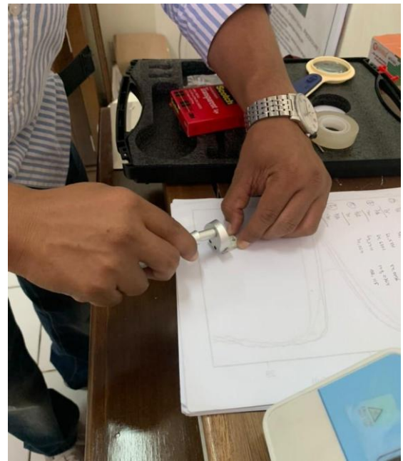
Fig.6. Cross-cut adhesion test of the HA coating.
