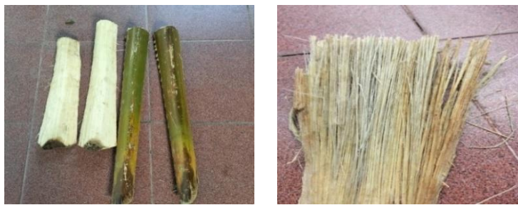
Fig. 2. (a) Palm fronds, (b) fiber from fronds.
