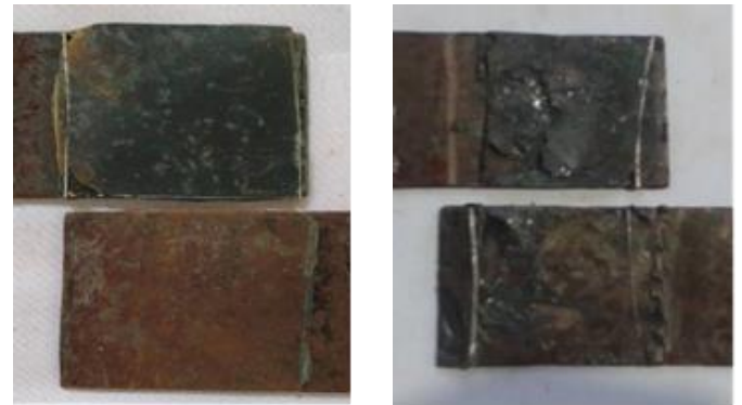
Fig. 5. Fracture of the epoxy adhesive bonding (AB) specimens.
