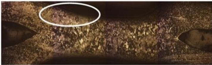
Fig. 9. The identified surfaces defect of the hybrid spot welding-epoxy adhesive (SWAB) A90 T10 specimen.
