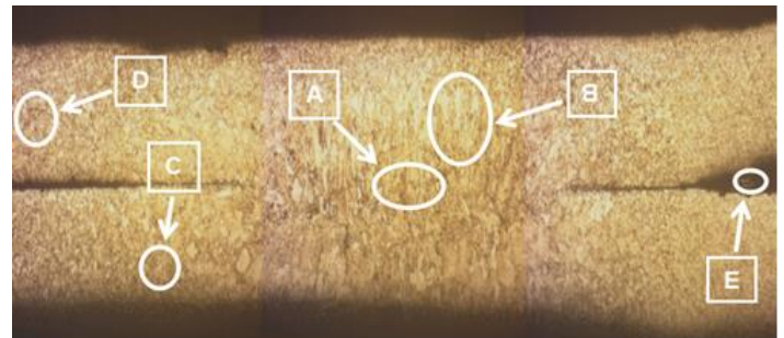
Fig. 7. Observation of the macrostructure of the spot welding-epoxy adhesive (SWAB) A90 T06 specimen.
