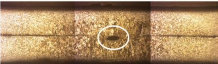
Fig. 10. A defect void of the hybrid spot welding-epoxy adhesive (SWAB) A05 T06 specimen.
