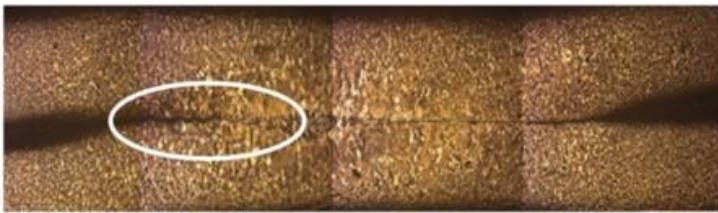
Fig. 8. The crack defect in the hybrid spot welding-epoxy adhesive (SWAB) A90 T02 specimen.
