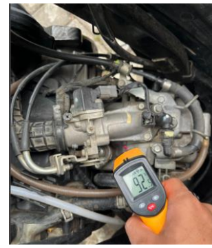
Fig. 1. The engine temperature test is performed by measuring the engine temperature with a thermogun.
